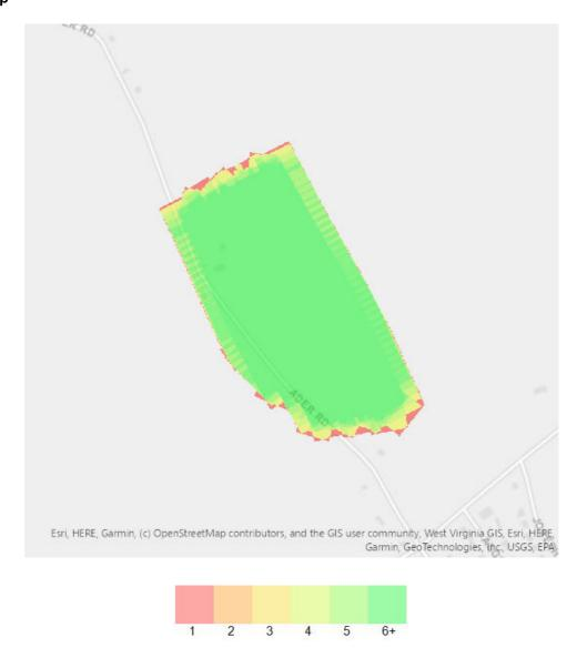
The amount of overlap between image projections after processing. Areas with high overlap produce the most accurate results. Avoid placing control points in areas of low overlap, as this could affect their accuracy.
