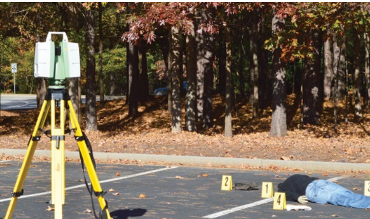
A mock crime scene demonstrates the use of a laser scanner to quickly and accurately capture all the details of the scene
