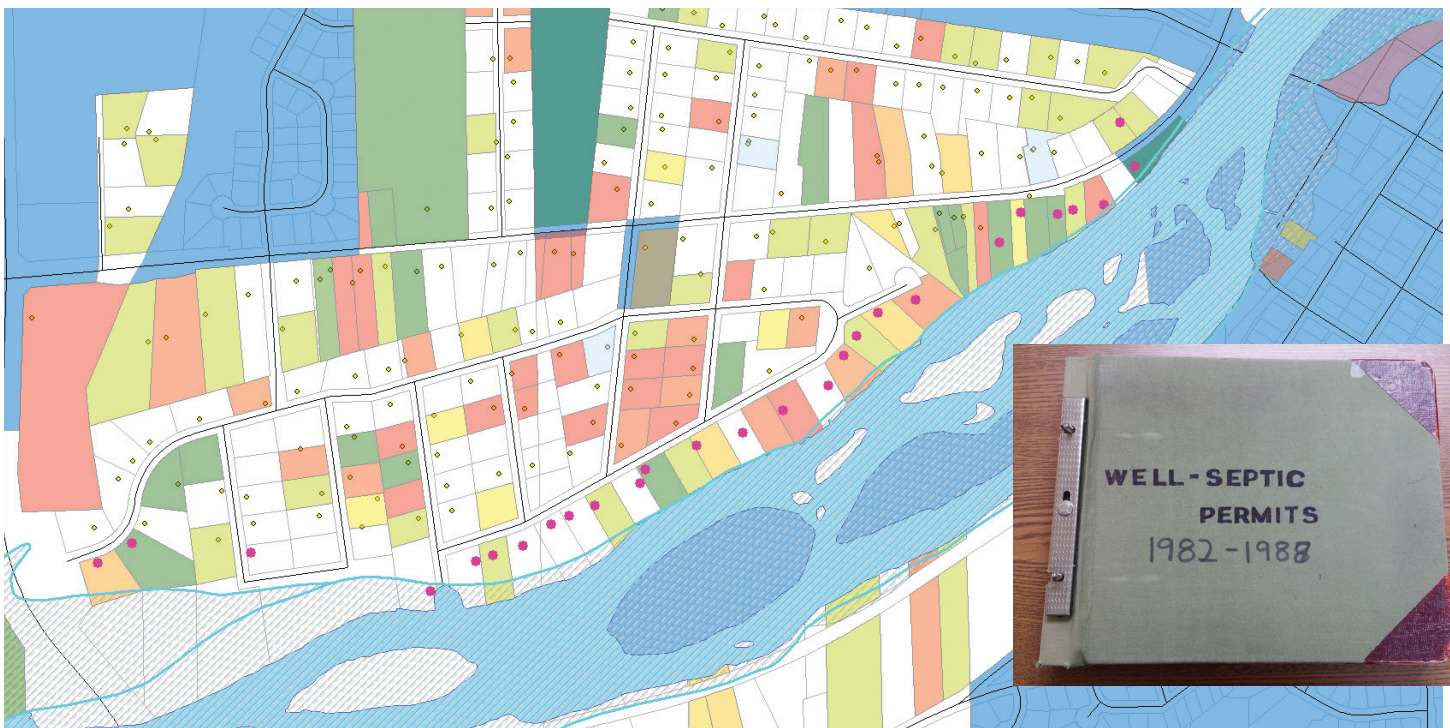
↑ The round points visible in this image are private water well locations. The darker points are private water wells located within a 250' buffer of the Fox River. KCHD worked closely with the county GIS coordinator after a recent flood event to develop ways to identify wells that are at or near the known flood elevation. Inset Right: Example of an old Permit Record Book. These were in use until 2001.
