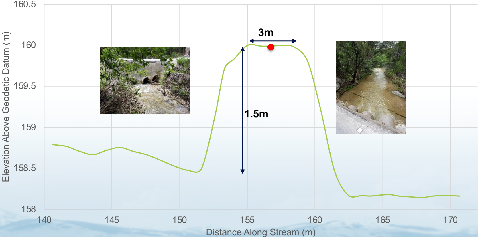
Stream Profile at Low Water Crossing
